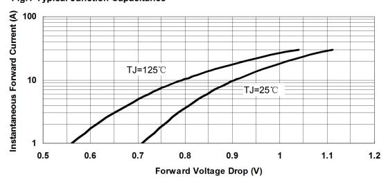
Fig.3-Typical Instantaneous Forward Voltage Characteristics
